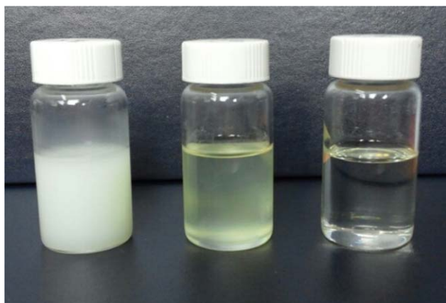
Figure 2. Status of the macropolymers: (a) wax-like (entry 1 in Table I), (b) turbid oil (entry 5 in Table I), and (c) clear oil (entry 2 in Table III). [Color figure can be viewed in the online issue, which is available at wileyonlinelibrary.com .]
